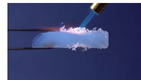
Mica materials for fire spread prevention prevent an ignited cell from affecting adjacent cells.
