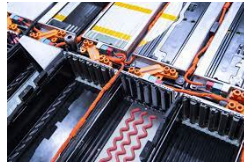
Lithium-ion batteries with mica materials for fire spread prevention
