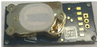
There are three connections to the sensor using 3 pin thru hole connector. Pin1 (V+ = 9-16VDC) is designated by the square pin pad. Pin 2 (LIN) is the center pin. Pin 3 (GND) is opposite the square pad.
