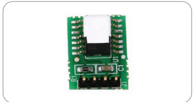
Replaceable, humidity sensor. Specially designed hydrophobic filter to prolong sensor calibration life.
