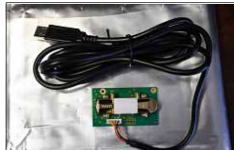
Figure 6: T6613/6615 CO 2 Sensor Connected to USB Cable
