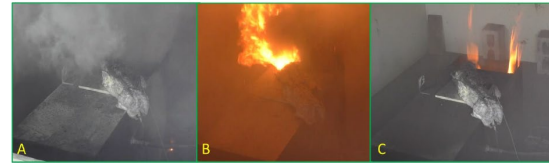
Figure 82: Mid-test, NMC (Bolt), ABC powder (A: ABC powder deployed, B: first re-ignition, C: second re-ignition)
