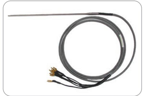
The **Thermometrics Type S/AS/ES** temperature standards consist of ultra-stable thermistor probes assembled into thin wall stainless steel housings with shielded extension leads. The thermistors used receive special processing to ensure long term stability. All thermistor temperature standards are ruggedly constructed and are suitable for liquid immersion.
