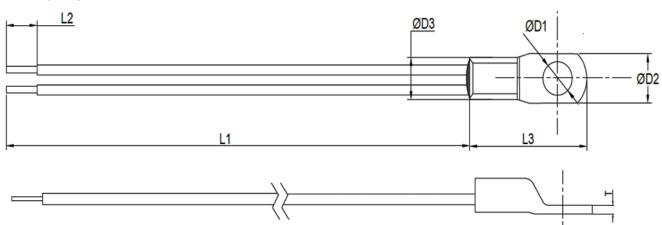
Coding: Eyelet size and wire length are specified by product code - RTS203C1R5M3L501
