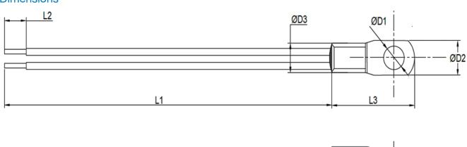
Coding: Eyelet size and wire length are specified by product code -
